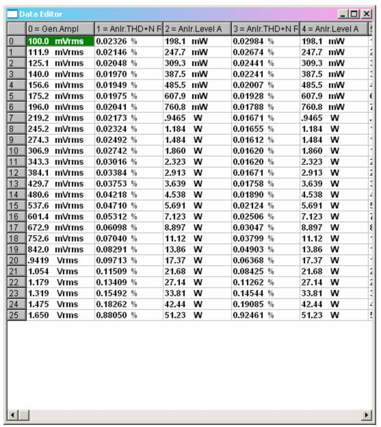
THD vs LEVEL AT 2KHz BOTH CHANNELS DRIVEN INTO 8 OHM
