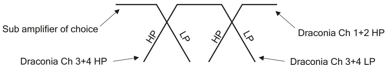
Note that when Draconia is configured this way, it is only part of the tri-amplified system. It only performs the high pass and bandpass/midrange functions in a TWO CHANNEL FORMAT.
