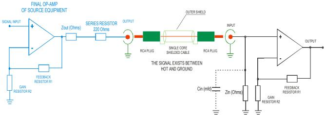
The op-amp of the source equipment is at the left side. It has an output impedance of Zo and in series we have added a 220 ohm resistor (typical) which isolates this op-amp from the capacitive loading effects of the cable AND the input capacitance of the receiving equipment. I have lumped these together as "Cin".
