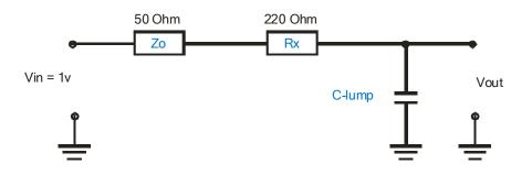
In the case of the 1 metre cable, C-lump is 50pF + Cin (say 220pF) = 270pFC-lump forms a potential divider with the 270 ohm resistors. The capacitive reactance of C-lump (C) is Xc = 1/6.28 x F x C.
