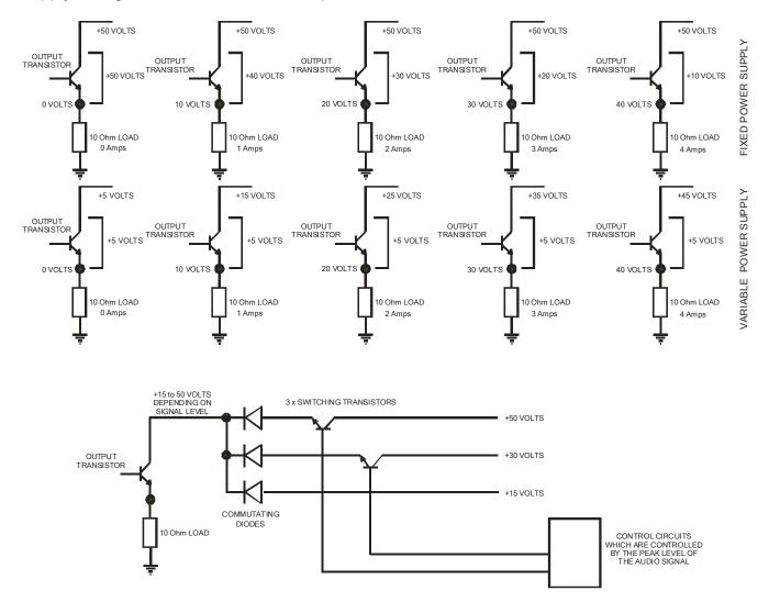
Let us examine the above diagrams. A single transistor shown for simplicity but the bottom half of the output stage is a symmetrical PNP transistor
