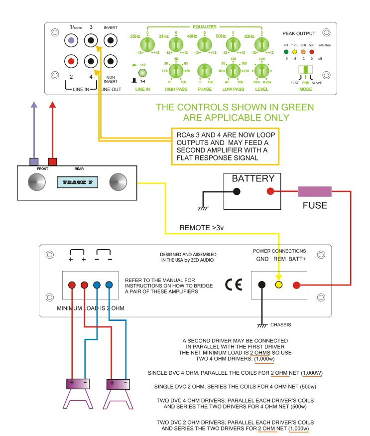
MINOTAUR driving one or more speakers as a stand alone amplifier from a four output signal source and set to FLAT mode. This drawing applies to any configuration where a single MINOTAUR is used.
