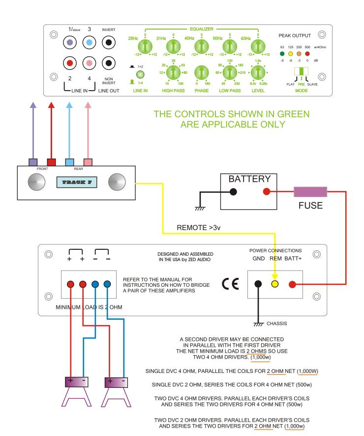
**MINOTAUR** driving one or more speakers as a stand alone amplifier from a two output signal source.
