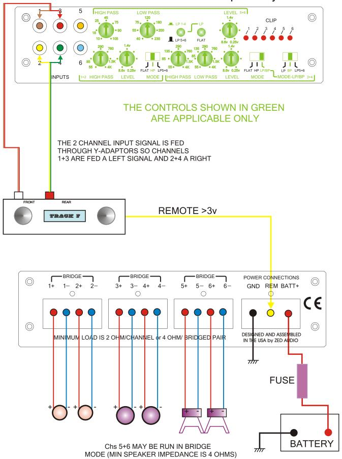
**LEVIATHAN** jumper links to parallel the inputs instead of using external Y-Adaptors.
